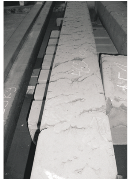
Fig. 15: Bar out of 1.4452-material with edge cracks. Root cause: precipitation of nitrogen pearlite due to nitrogen pick-up in the surface area of ~ 1.3 % N
