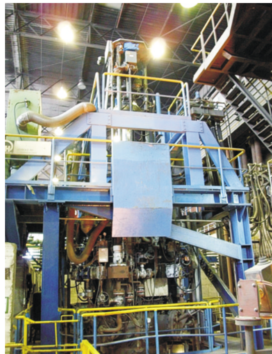
Fig. 5: View of the industrialized P-ESR process for ingot weight up to 20 t und \varnothing 1030 mm
